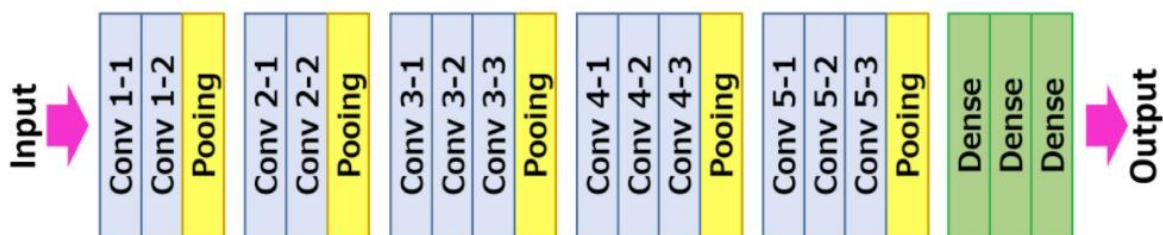
Figure 3 - Architecture of VGG16
